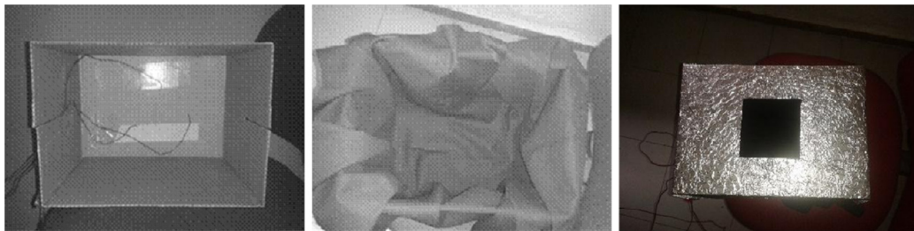
Fig. 4. Left: The hollow target (a simple card box for a commercial product; the three placed thermocouples are also shown), Centre: the black coloured textile covering the internal surface of the hollow target and Right: the reflective surface on the box cover as the auxiliary set up is assembled and ready for use.
